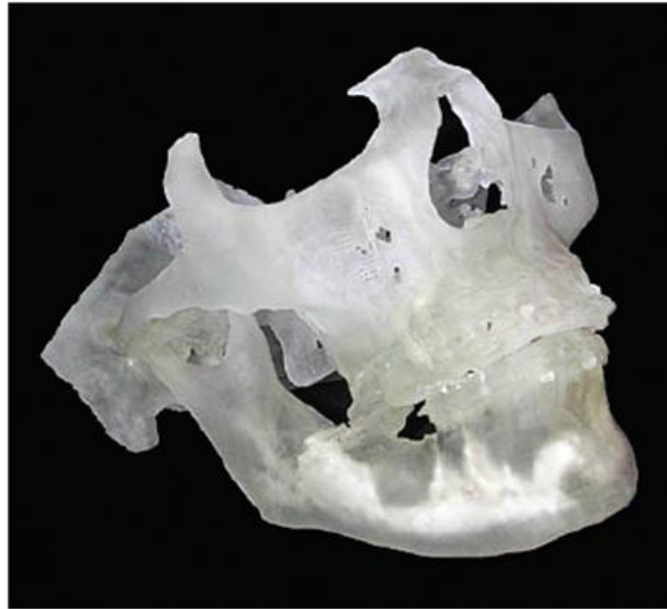
Figure C2: Physical prototype made using stereo lithography
