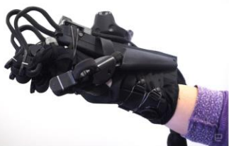
This haptic glove, the AxonVR , uses micro-pockets of air in the touch surfaces to communicate touch to the user.
