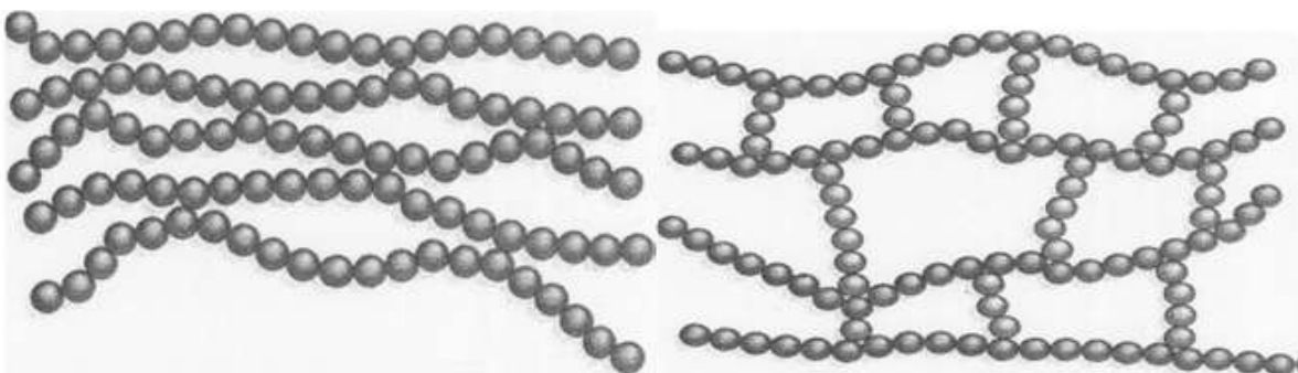
Left hand diagram above – thermoplastic macromolecules
