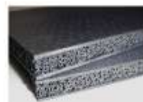
Carbon/silicon carbide (C/SiC) fabric used to reinforce ceramic matrix composite face sheets - creates a sandwich structure capable of withstanding high-heat flux environments - ideal for aerospace vehicles
