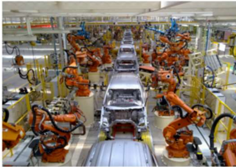
Figure C6: Welding robots in automotive production ABB Robotics AB, Västeras, Sweden
