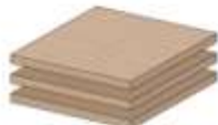
Exploded view showing that grains of subsequent layers of veneer are laid at 90° to each other
