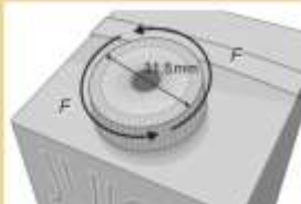
Figure 4: Dimensions of the screw cap and indication of the direction of force applied
